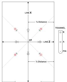
Measure the room to be laid, in both directions, including any alcoves etc.
